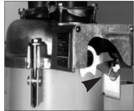
Figure 3. The non-reclosing feature is set with a handle under the sleet hood (see arrow). When the handle is down (left), the recloser will trip on overcurrent and lock out without reclosing. When the handle is up (right), the recloser will operate according to its internally set program.
